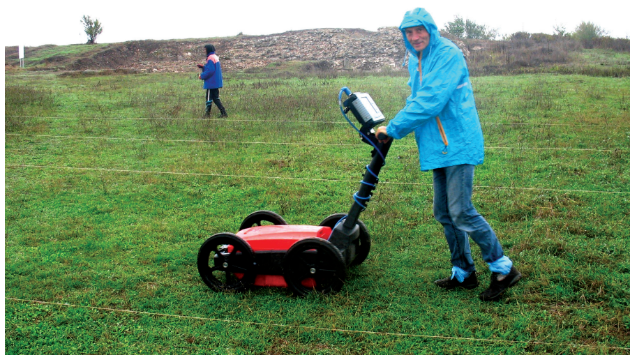
Figure 4. Geophysical survey in Deultum with ground penetrating radar. (Photo: Lyudmil Vagalinski).
