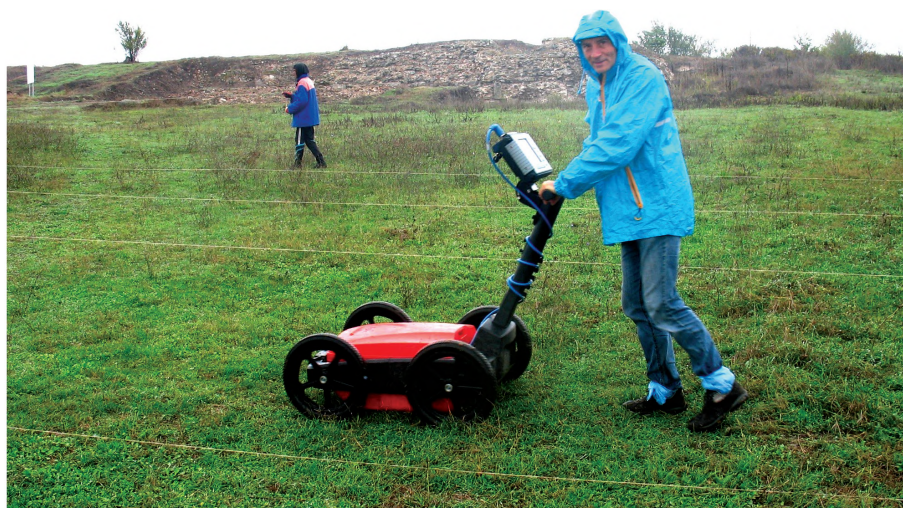
Figure 4. Geophysical survey in Deultum with ground penetrating radar. (Photo: Lyudmil Vagalinski).
